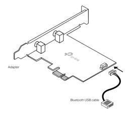
3. Locate an available PCIE X1 slott (X1, X4 or X16) and carefully insert the adapter.
